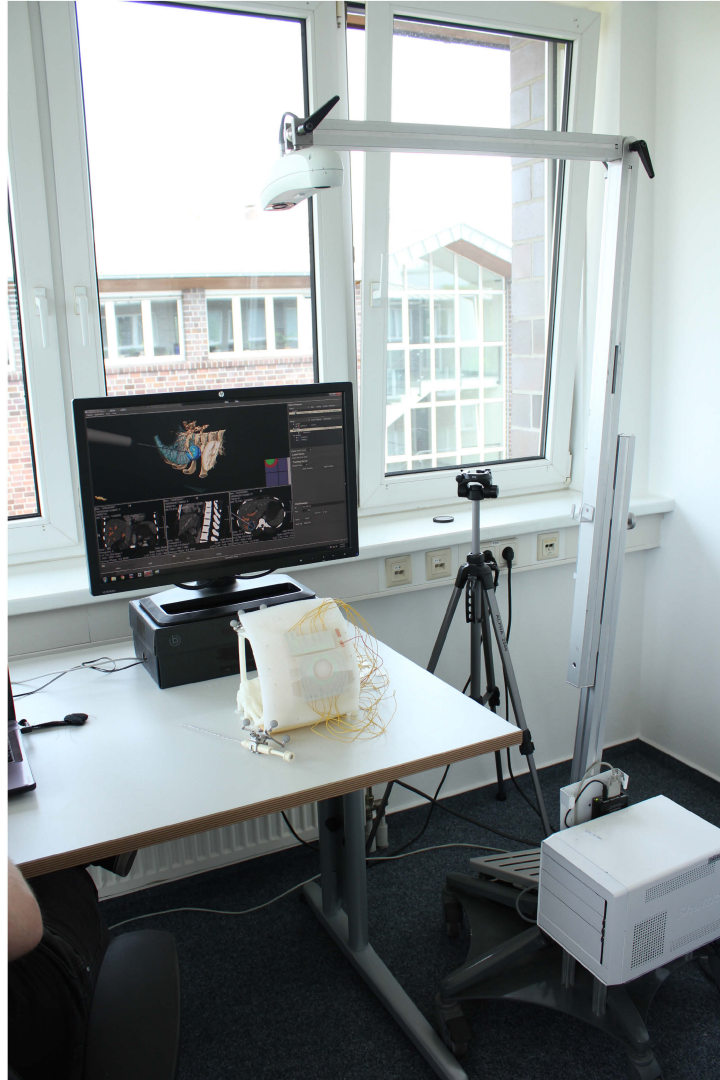
Fig. 6. Overview of the evaluation setup. The phantom is fixed on a table with a black box behind it that hides the controlling electronics and a computer monitor on top. The scene is tracked from above with an optical medical tracking system.
